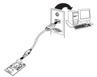
3. If using an RS-232 connection, connect the serial interface cable to the engine and to the matching port on the back of the computer.
